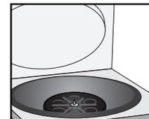
With door and rotor lid open, rotor is ready to be loaded.
