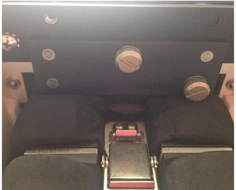
Once the 1405F or 1405DF is installed in the enclosure, environmental shelter or other weather proof temperature controlled environment, you will need to place the shipping bracket in its neutral position.
