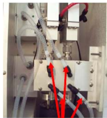
Valve to Chiller Tubing
