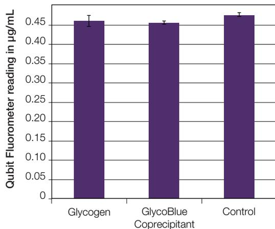
**Figure 3.** Results from the Qubit dsDNA BR assay for samples containing DNA plus 25 ng/ $\mu$ L glycogen or GlycoBlue Coprecipitant (in the assay tube) compared to samples containing DNA only. The DNA concentration in the assay tubes was 0.5  $\mu$ g/mL (near the low end of the Qubit dsDNA BR assay range). Assay tubes contained between 10  $\mu$ L and 15  $\mu$ L of sample; results are the averages of two or three replicates.
