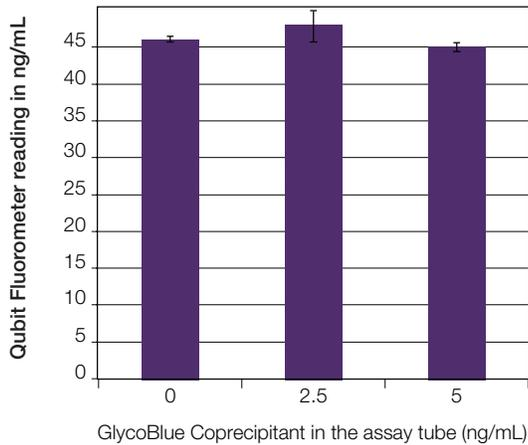
**Figure 9. Results from the Qubit RNA HS assay for samples containing RNA plus 0–5 ng/μL GlycoBlue Coprecipitant (in the assay tube).** The RNA concentration in the assay tubes was 50 ng/mL (near the low end of the Qubit RNA HS assay range). Note that the results obtained in the presence of 0 to 5 ng/μL GlycoBlue Coprecipitant are within 5% of the control readings. Assay tubes contained between 10 μL and 15 μL of sample; results are the averages of two replicates.
