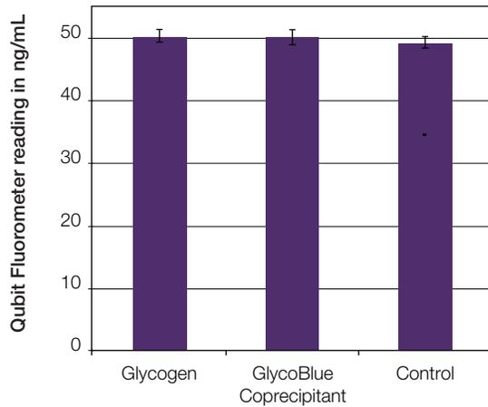
**Figure 1.** Results from the Qubit dsDNA HS assay for samples containing DNA plus 25 ng/ $\mu$ L glycogen or GlycoBlue Coprecipitant (in the assay tube) compared to samples containing DNA only. The DNA concentration in the assay tubes was 50 ng/mL (near the low end of the Qubit dsDNA HS assay range). Assay tubes contained between 10  $\mu$ L and 15  $\mu$ L of sample; results are the averages of three replicates.
