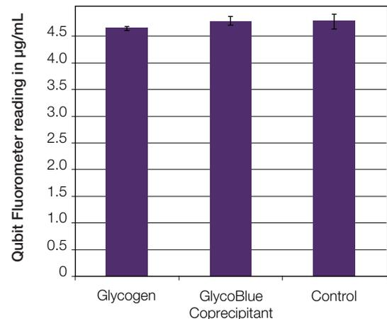
**Figure 4.** Results from the Qubit dsDNA BR assay for samples containing DNA plus 25 ng/ $\mu$ L glycogen or GlycoBlue Coprecipitant (in the assay tube) compared to samples containing DNA only. The DNA concentration in the assay tubes was 5  $\mu$ g/mL (near the high end of the Qubit dsDNA BR assay range). Assay tubes contained between 10  $\mu$ L and 15  $\mu$ L of sample; results are the averages of three replicates.
