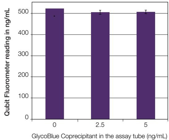
**Figure 10. Results from the Qubit RNA HS assay for samples containing RNA plus 0–5 ng/μL GlycoBlue Coprecipitant (in the assay tube).** The RNA concentration in the assay tubes was 500 ng/mL (near the high end of the Qubit RNA HS assay range). Note that the results obtained in the presence of 0 to 5 ng/μL GlycoBlue Coprecipitant are within 5% of the control readings. Assay tubes contained between 10 μL and 15 μL of sample; results are the averages of two replicates.
