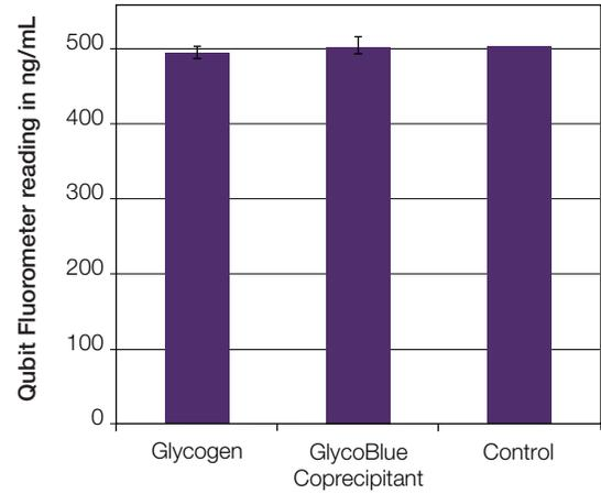
**Figure 2.** Results from the Qubit dsDNA HS assay for samples containing DNA plus 25 ng/ $\mu$ L glycogen or GlycoBlue Coprecipitant (in the assay tube) compared to samples containing DNA only. The DNA concentration in the assay tubes was 500 ng/mL (near the high end of the Qubit dsDNA HS assay range). Assay tubes contained between 10  $\mu$ L and 15  $\mu$ L of sample; results are the averages of three replicates.
