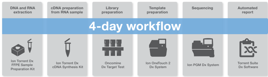
Figure 2. The Oncomine Dx Target Test utilizes a single streamlined NGS workflow for detecting cancer-associated biomarkers, incorporating reagents, instrument systems, and bioinformatics. The turnaround time from FFPE sample to report is 4 days.
