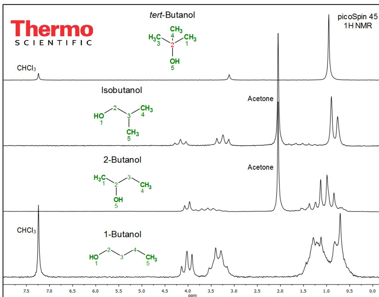
**Figure 1.** Full experimental <sup>1</sup>H NMR (45 MHz) spectra of, from top to bottom, *tert*-butanol, isobutanol, 2-butanol and 1-butanol.
