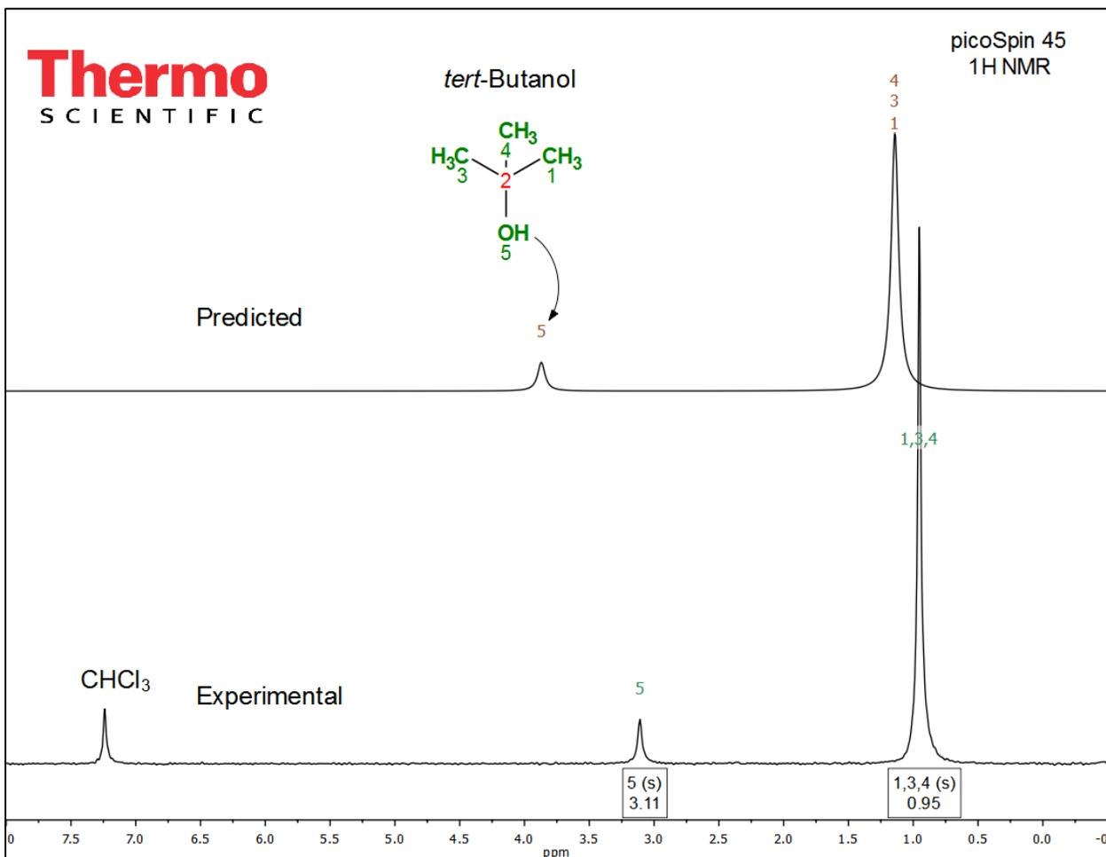
**Figure 6.** Full experimental (bottom) and predicted (top) <sup>1</sup>H NMR (45 MHz) spectrum of *tert*-butanol in CHCl<sub>3</sub> (50:50 v/v).
