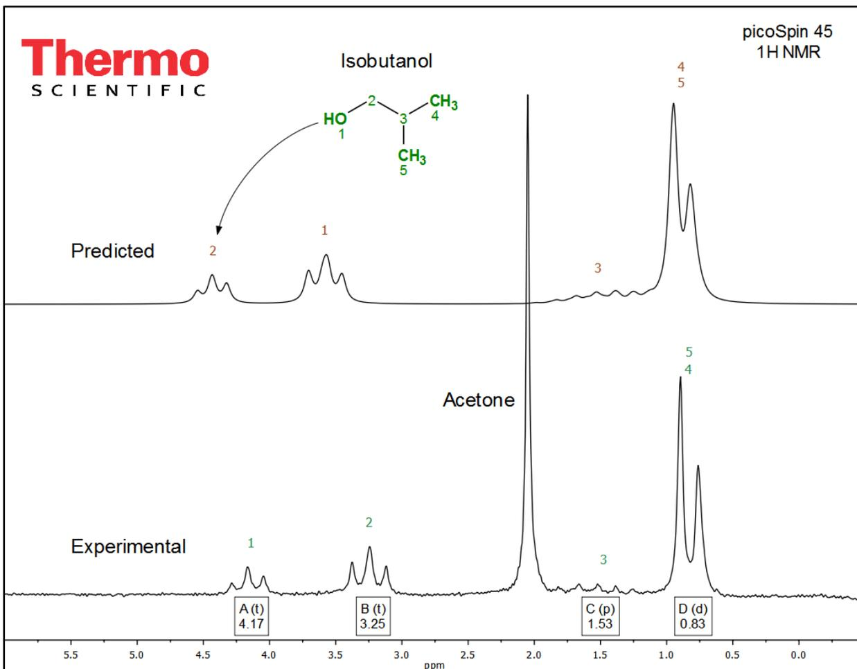
**Figure 5.** Full experimental (bottom) and predicted (top) <sup>1</sup>H NMR (45 MHz) spectrum of isobutanol in acetone (50:50 v/v).
