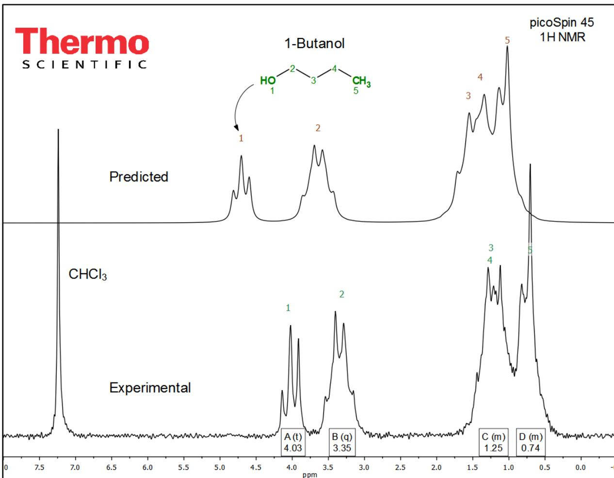
**Figure 3.** Full experimental (bottom) and predicted (top) <sup>1</sup>H NMR (45 MHz) spectrum of 1-butanol in CHCl<sub>3</sub> (50:50 v/v).
