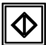
This key is used to start the wash or spin run. The indicator to the left of this key will light when the RUN key is pressed, indicating that the instrument is in the run mode.
