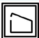
This key is used to power the cover solenoid and open the cover. The indicator to the left of this key will light whenever the Power Switch is in the On position and the rotor is stopped. Press the OPEN COVER key to release the cover.
