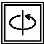
This key is used with the appropriate number (0 through 9) key(s) to use the Cell Washer as a centrifuge at 2800 rpm (50 Hz) or 3400 rpm (60 Hz) in a timed (from 1 to 999 seconds) run or in an untimed run using the HOLD key. The indicator to the left of this key lights when the SPIN key is pressed indicating that the unit is in the spin mode.
