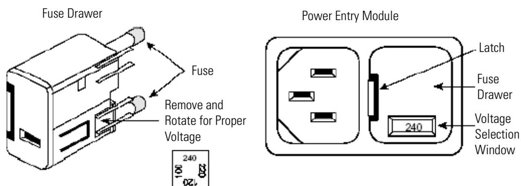
1. Locate the power entry module on the back side of the unit. The removable fuse drawer is located in the module. A small latch holds the drawer in place. Press this latch, then slide the drawer out.
