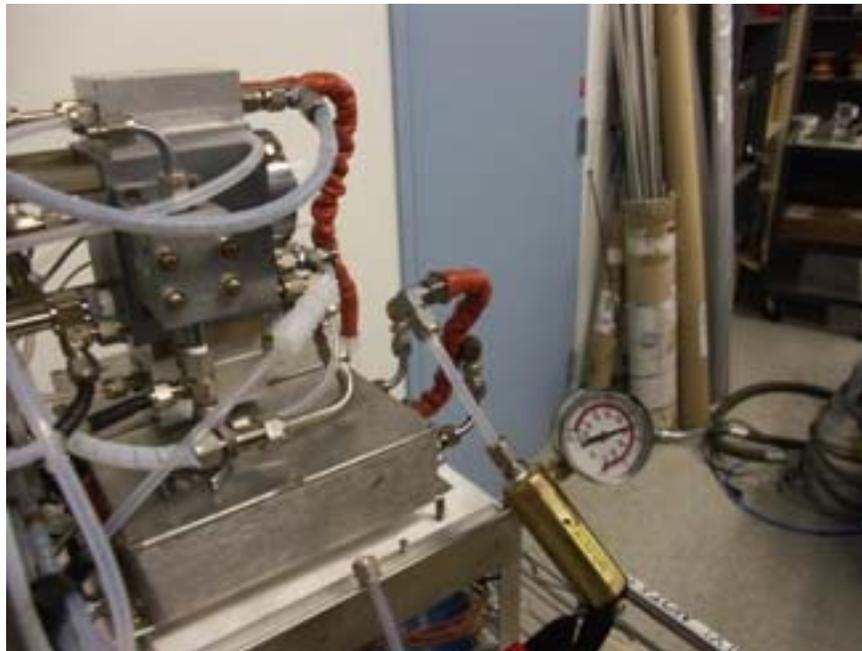
14. Ensure the teflon line at the orifice block are not melted or leaking.
