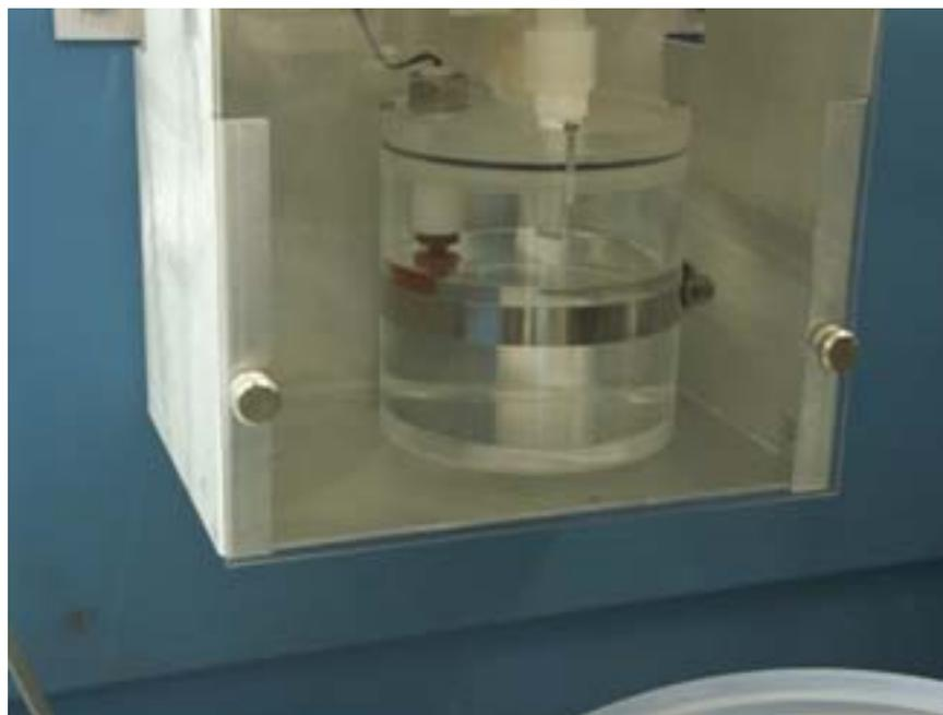
10. Disconnect 3/8 cal line from the outlet bulkhead of the hydrator, put the system in System Span mode, call up the 81 pressure diagnostic screen, and place your thumb over the hydrator outlet. The pressure on the 81i should quickly (~4 seconds) peg out to >1220. Y/N (**do not plug for more than 15 seconds or this may result in the 81 being over pressurized**). Reconnect tubing.
