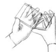
Figure 7a and 7b. Opening the cassette to expose the gel.
