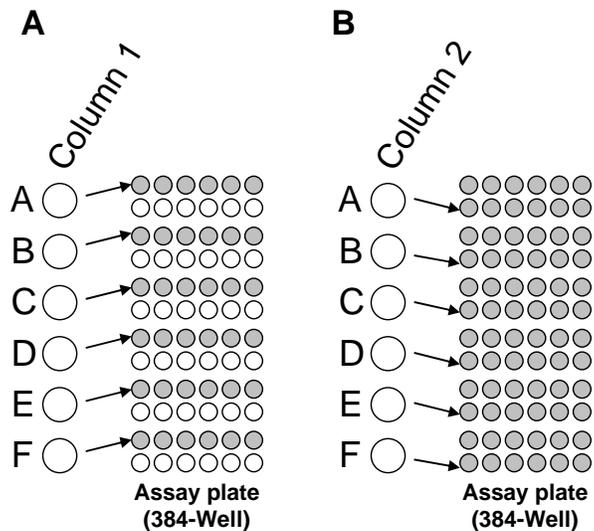
2. Add 4  $\mu$ L of competitor solution to three wells for each tracer concentration (columns 1–3).
