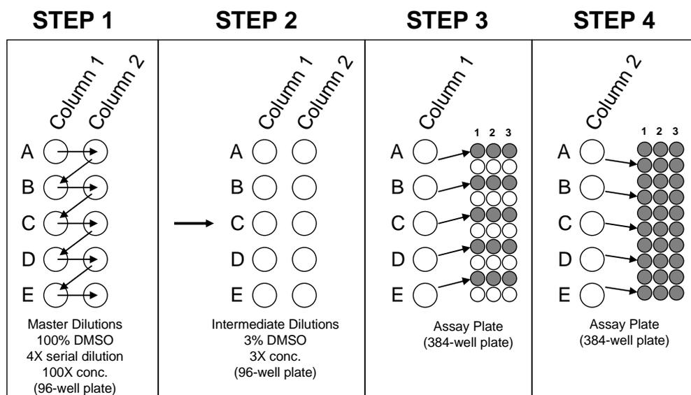
2. Dilute the “Master Dilution” series 25-fold into Kinase Buffer A. Remove 5 µL of each concentration of diluted compound, transfer to another 96-well plate, add 125 µL of Kinase Buffer A and mix (Figure 6, Step 2).
