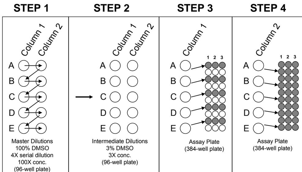
2. Dilute the “Master Dilution” series 25-fold into Kinase Buffer A. Remove 5 μL of each concentration of diluted compound, transfer to another 96-well plate, add 125 μL of Kinase Buffer A and mix (Figure 6, Step 2).
