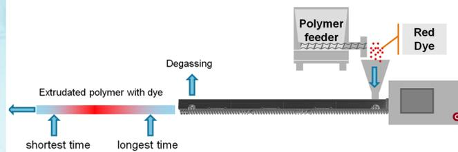
FIGURE 1: Set up of screws and barrel used for the scale up experiments on the Pharma 16. At the feeding section the Kollidon® VA64 is added as well as the pigment is added at a given time  $T_0$ . The degassing section at the left hand side is an atmospheric degassing to allow water vapor to evaporate out of the polymer
