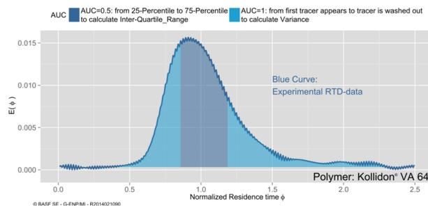
FIGURE 2: Residence time distribution of Kollidon® VA 64 in the Pharma 16 Extruder with a feed rate of 2 kg/h, a screw speed of 200 rpm and a barrel temperature ramp up to 260°C.
